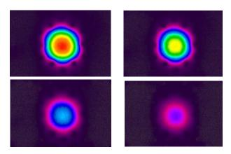
Figure 2: Near-field images of the fiber for optimum alignment (A) and gradually misaligned input beam (B-D). The output beam symmetry is maintained for all positions of the input beam and no higher order modes could be excited. The mode field diameter is 32  $\mu m$ . The images are obtained on a CCD camera.
