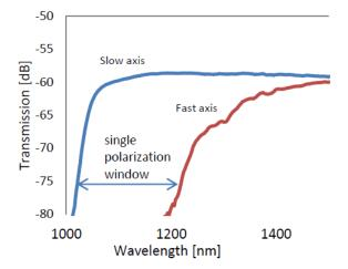
Figure 6: Transmission scan for the two polarization directions. The polarizing fiber structure yields a strong attenuation for the fast axis (y-polarization) for wavelengths <1200nm, while the slow axis (x-polarization) is well guided down to <1000nm.
