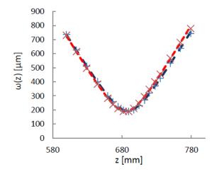
Figure 5: Measured spot size vs. propagation distance for a collimated beam from a DC-200/40-Pz-Yb fiber. The spot size was measured both in x-direction and y-direction. The fits yield an  $M^2$  value better than 1.15.
