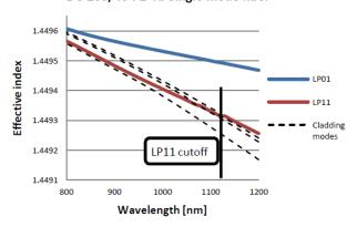
Figure 3: Simulated effective mode indices of the first 5 modes in a DC-200/40-PZ-Yb fiber. The LP11 mode exhibits a short-wavelength cutoff at ~1120nm, and the fiber is single mode for wavelengths below. The figure refers to the transverse (x-) polarized modes. The stress applying parts induce a strong birefringence, which lowers the effective indices of the corresponding y-polarized modes, which therefore are not guided in the wavelength range shown.
