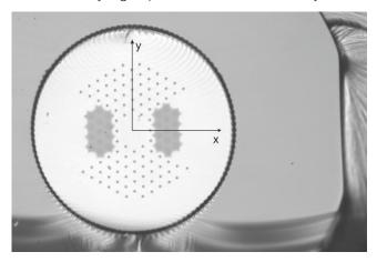
Figure 1: Fiber cross-section showing the microstructure, stress applying parts, air cladding and polished outer cladding sides.
